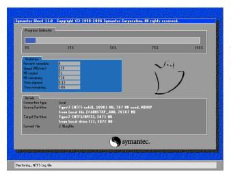
When the machine is turned off, plug the U disk into the USB port behind the host, and the U disk will restore after the machine restarts. As shown in the figure, the system is restoring, and it needs about 20 minutes.
