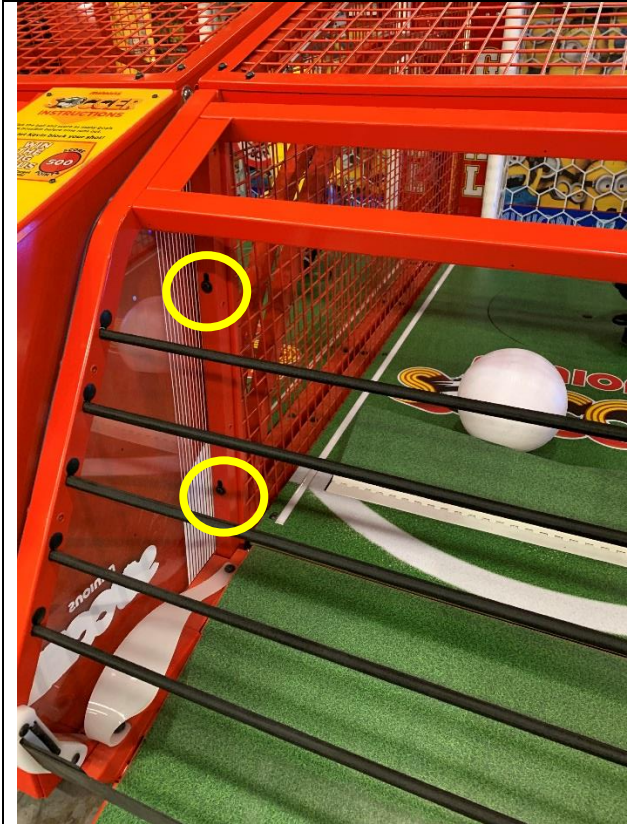
Bolt the console section onto the Main Playfield section
