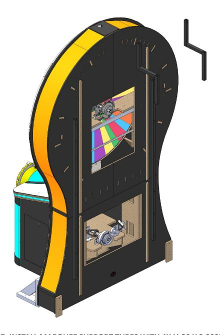
STEP 7: INSTALL MARQUEE SUPPORT TUBES WITH 4X 1/4-20 X 2.000L SCREWS
